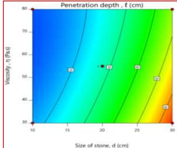
Figure 3. 4- Diagram of relationship between penetration depth and cavity size and viscosity, 2D format
