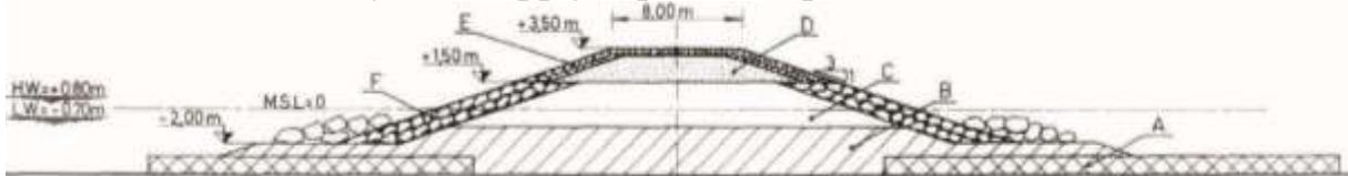
Figure 1.4- Typical section of Hook-Netherlands breakwater [30]
