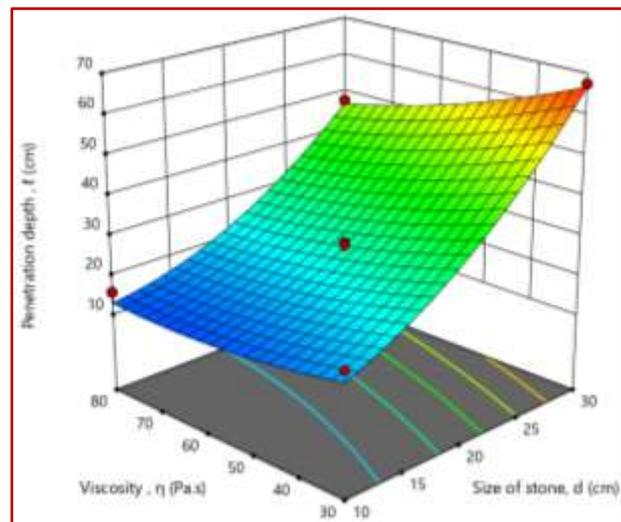
Figure 3. 5- Diagram of relationship between penetration depth and size of the rock and viscosity, 3D form
