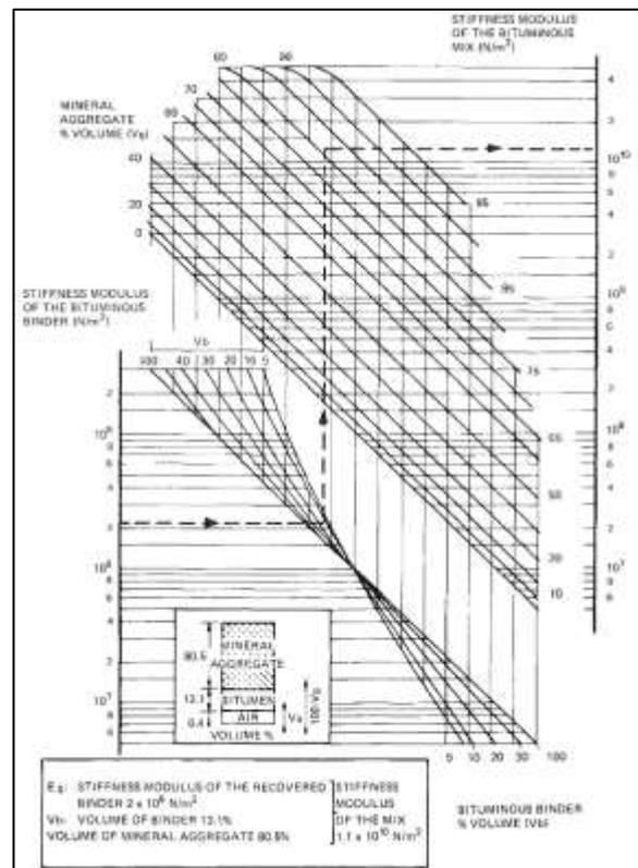
Figure 1.13- Diagram for estimation of hardness modulus of VLHH with bitumen [17]
