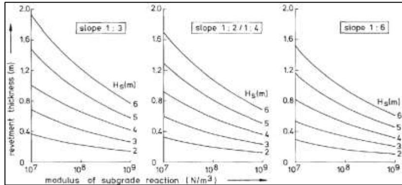
Figure 4. Relationship of thickness, dyke jet and standard wave height, dyke tilt for reinforcement layer made of the grouting mortar mixture material [31]
