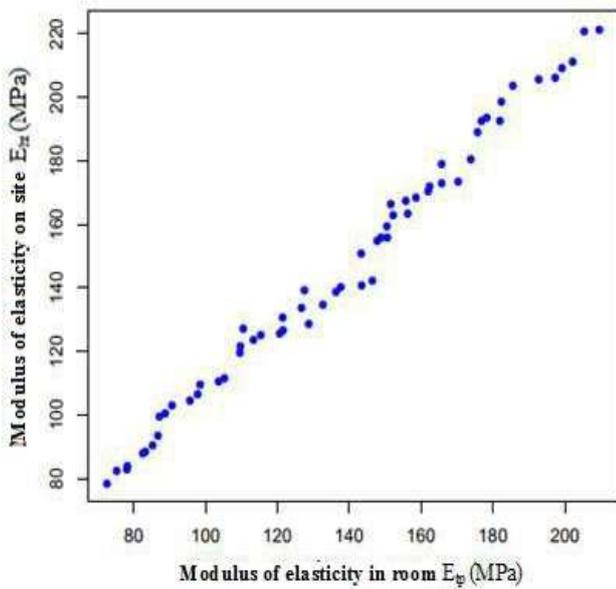
Figure 3. 20 - Scatter diagram between  $E_{ht}$  and  $E_{tp}$
