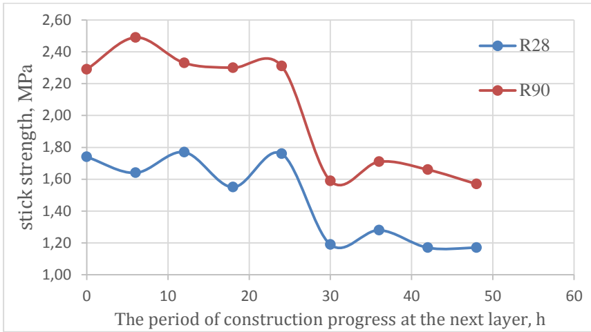
Picture 3.13. Figure is shown the strength of tension at between old and new layers of RCC used admixtures MINERAL CHEMICAL ADMIXTURE ADVA 181
