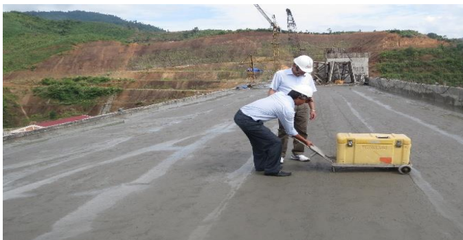
Picture 4.6. Testing Volume Density for RCC after compacting
